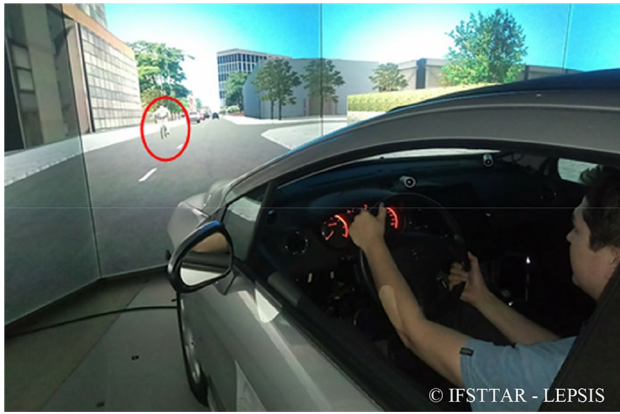
Fig. 1 The car driving simulator used and an example, indicated by a red circle, of one of the cyclists to be detected by the participants (Color figure online)
