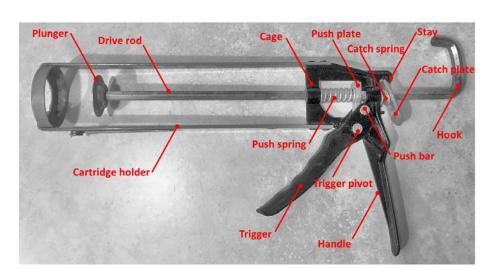
The example of a manual caulking gun (Figure 1) will be used to illustrate the proposal being put forward in this chapter.
