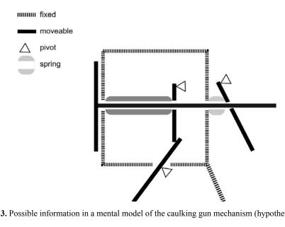
Fig. 3. Possible information in a mental model of the caulking gun mechanism (hypothetical)
