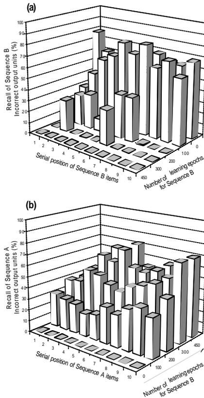
Figure 3. Catastrophic forgetting in an SRN during multiple sequence learning. (a): Learning of sequence *B* (after having previously learned sequence *A*). By 450 epochs (an epoch corresponds to one pass through the entire sequence), sequence *B* has been completely learned. (b): The number of incorrect units for sequence *A* during learning of sequence *B*. After 450 epochs, the SRN has, for all intents and purposes, completely forgotten the previously learned sequence *A*.
